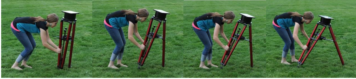
Figure 8: Extending the pier legs.
