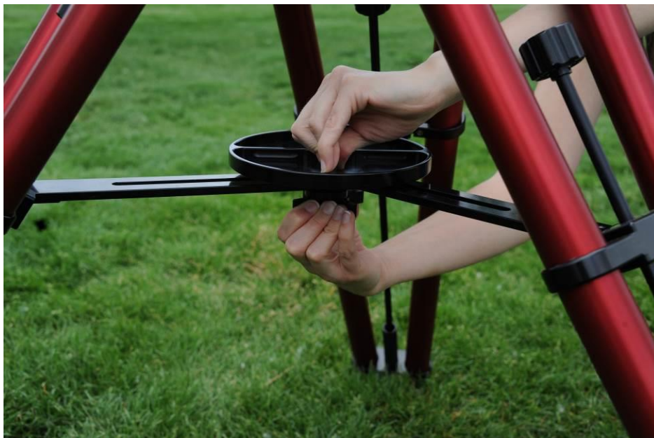
Figure 15: Loosen the clamp nut before collapsing the legs.
