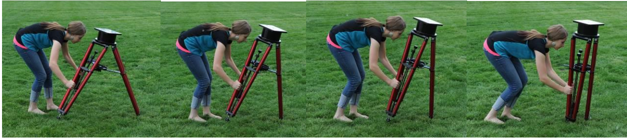
Figure 16: Photo sequence showing how to collapse the legs.
