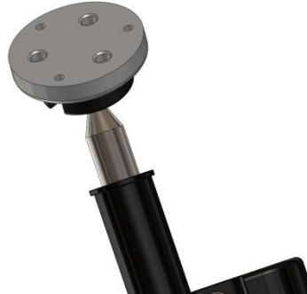
Figure 12: Tapped holes in pier feet.
